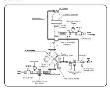
Suction pipe size should be at least the same diameter as the inlet connection size, even larger if highly viscous fluid is to be pumped. If suction hose is used, it must be of a non-collapsible reinforced type. Discharge piping should be of at least the same diameter as the discharge connection. It is critical,
